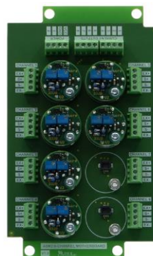
picture shows motherboard with 6 amplifiers
